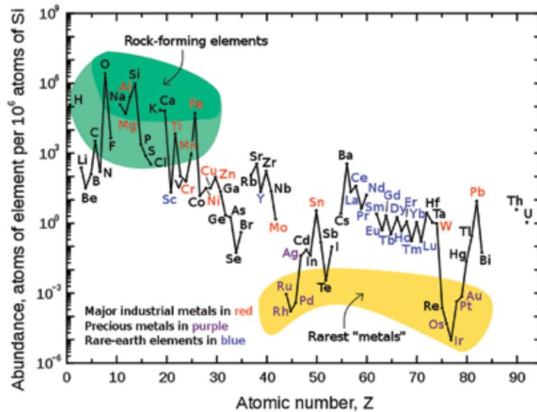
Figure 11: Abundance (atom fraction) of the chemical elements in Earth's upper continental crust as a function of atomic number.<sup>18</sup>
